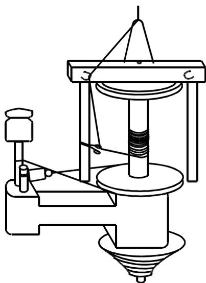
The brake band (tension cord) is crossed for clockwise spinning.
