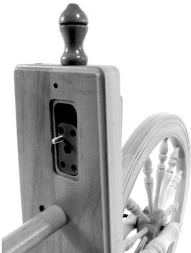
10) Tip the spinning wheel onto its front legs and wheel. Locate the maiden bar base into the table. Position the small barrel nut into the hole in the lower block and thread the drive belt tensioner into the barrel nut.
