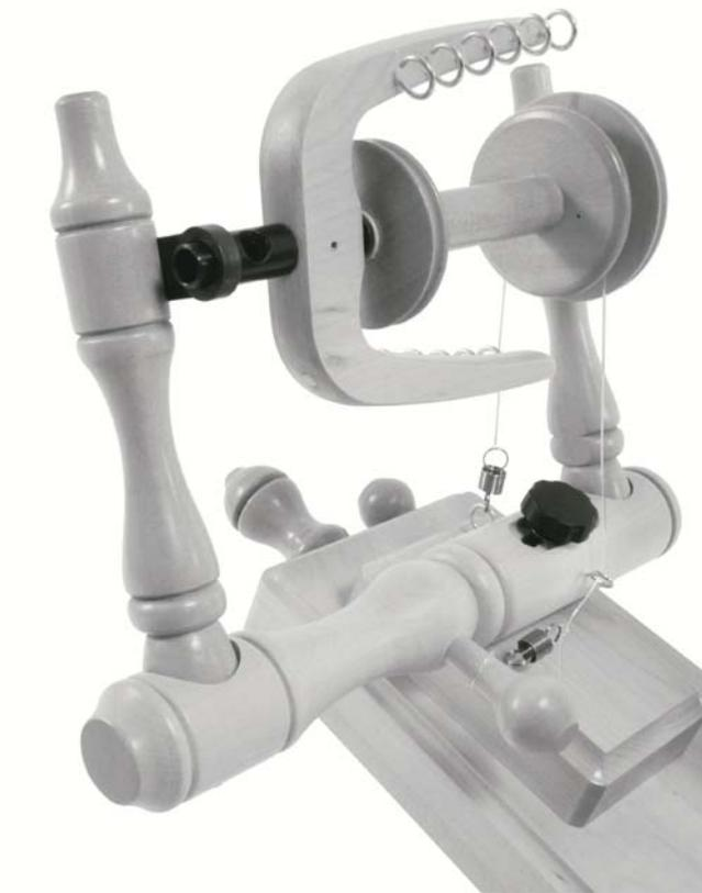
13) Wax the dowel ends then locate the two maiden uprights 'I' and 'J' into the maiden bar secure with 1 inch (25mm) pan head screws and small washers. Do not over tighten. When you have assembled your new wheel you may need to twist the uprights so they are 90° to the flyer shaft.
