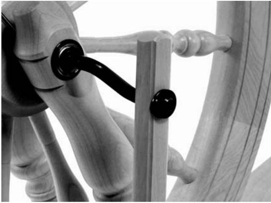
7) Secure the nylon flexible joint to the connecting rod 'H' with a 5/8 inch (16mm) pan head screw.
