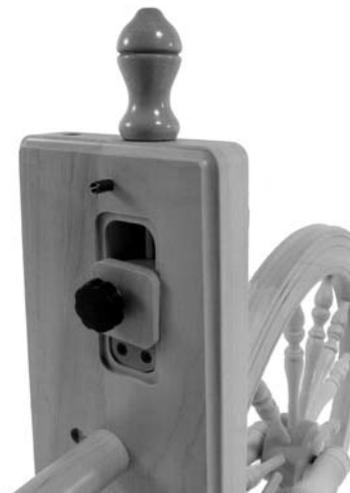
12) Wax the 1 3/4" (45mm) tension pin and insert it into the hole in the underside of the table to lock the drive belt tensioner in position. Leave 1/2" (10mm) protruding so it can be removed if necessary.
